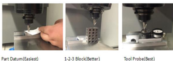
Figure 1: Methods of tool length offset in CNC milling machine
